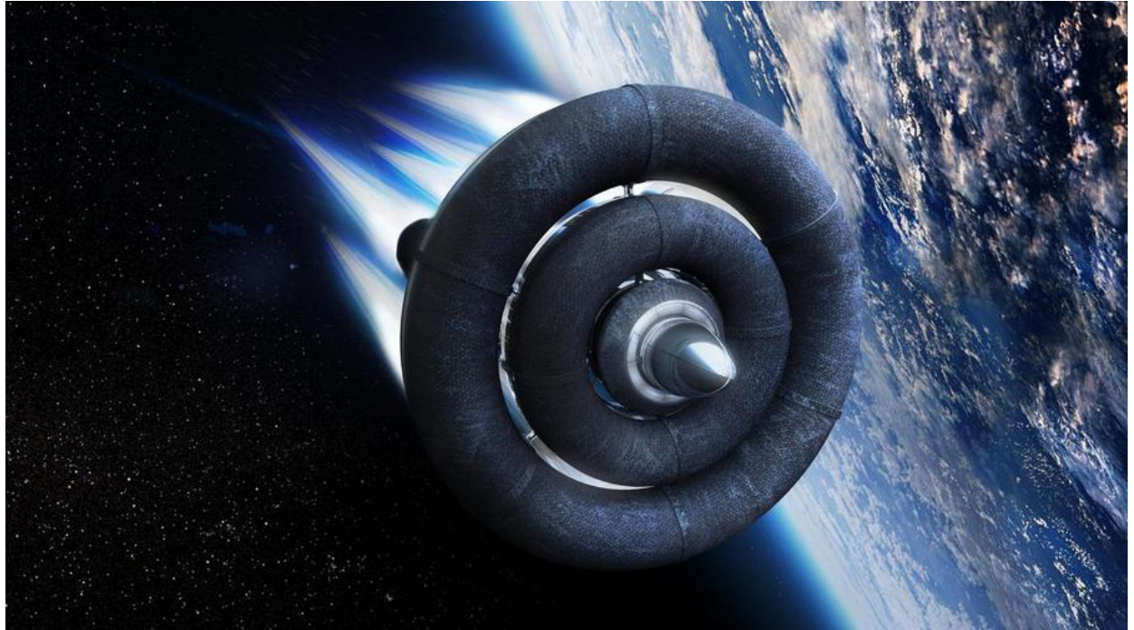
Artist's rendering of Bloostar after release from its balloon. Note the three nested stages and the payload in the center. (Source: Zero2Infinity)
