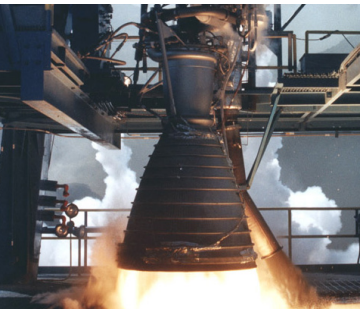
An RS-27A undergoing ground testing (ULA)
