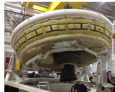
A STAR-48 motor used for NASA's Low-Density Supersonic Decelerator project (NASA)
