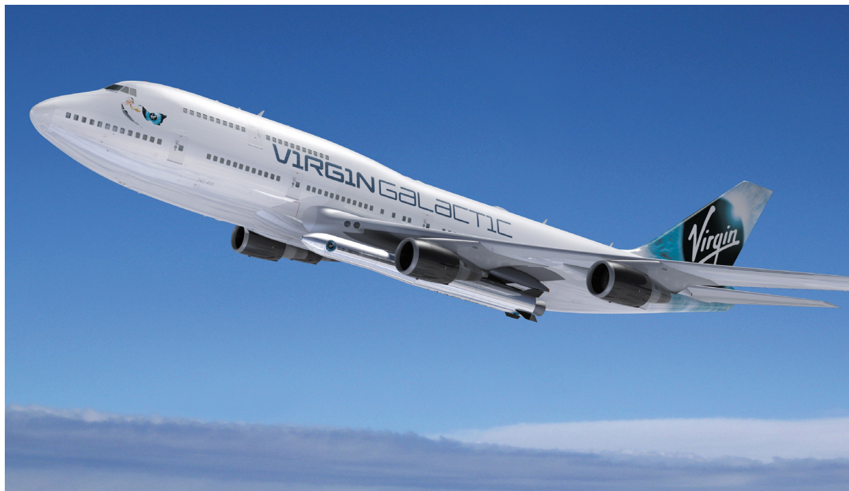
An artist's impression of the LauncherOne vehicle integrated with a Boeing 747-400 carrier aircraft. Source: Virgin Galactic
