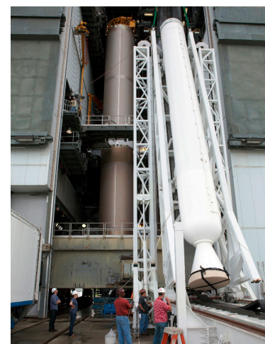
An AJ-60A being integrated with an Atlas V (Aerojet Rocketdyne)
